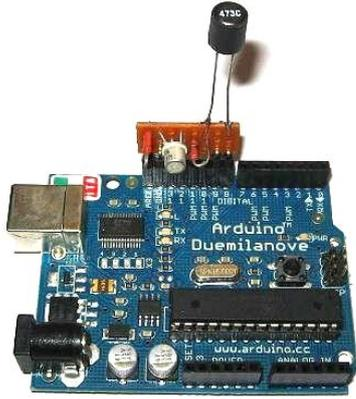
Fig. 5. Arduino Duemilanove board expanded with RFID tag simulation circuit.
